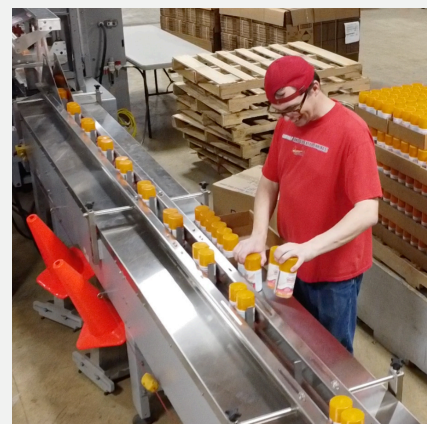
AEROSOL CAN AIR FRESHENERS ARE LOADED MANUALLY ONTO A CONVEYOR AND AUTOMATICALLY SHRINK WRAPPED TOGETHER IN PACKS.
